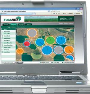
FieldNET's Map View feature uses GPS coordinates to let a grower view the status of all his pivots simultaneously
