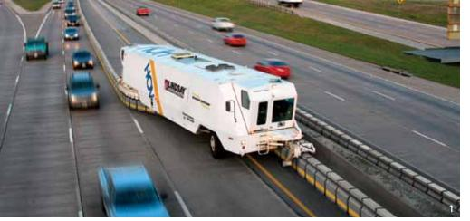
Road Zipper System updates include a new and innovative guidance system utilizing GPS and Ultrasonic technologies that enable the system to operate with great accuracy, minimizing the need for modifying existing infrastructure. Several other development projects were initiated in fiscal 2012 resulting in promising innovations for the future of moveable barrier technology.
