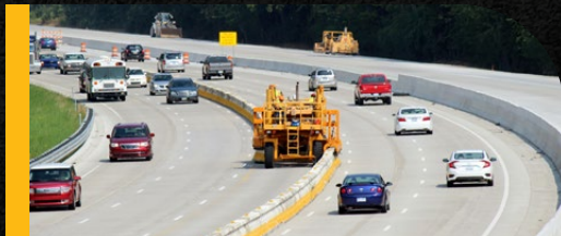
The Road Zipper System™ - Moveable barrier technology for maximum protection and flexibility to manage traffic and mitigate congestion
