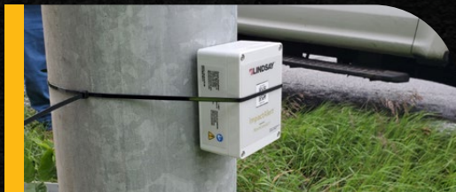
ImpactAlert™ - Real-time notifications and alerts for roadside asset impacts through the RoadConnect dashboard
