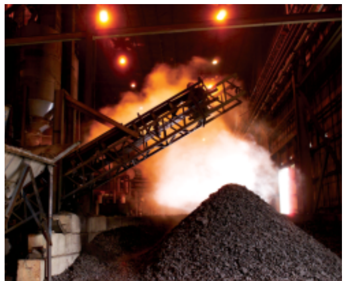
Hot-briquetted iron produced at Iron Dynamics is used in SDI's melt shop as a substitute for steel scrap and pig-iron ingots.
