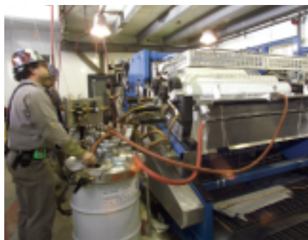
Top, left to right: Hot-rolling a steel slab to produce thin-gauge hot-rolled sheet steel in SDI's seven-stand hot mill; glowing flat-rolled steel is down-coiled onto a mandrel, from which it will be removed as a coil of steel—a hot band. Bottom, left to right: A view from the entry-end of Butler's new paint line, which is over 1,000 feet long; workers adjust the flow of paint to the rollers in the paint-application room; and various colors of painted coils, banded but not yet wrapped, await shipment.
