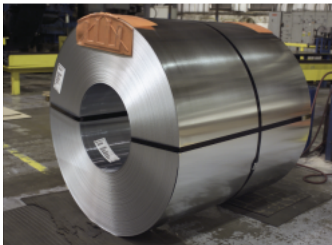
Left: A cold-rolled steel coil, banded for shipment. Such coils can be sold as is or galvanized (on Butler's Galv Line 2 or at SDI's newly acquired Jeffersonville galvanizing facility). Right: The final inspection and coiling station at the Jeffersonville galv line illustrates the new plant's highly automated equipment, similar to that used at Butler.
