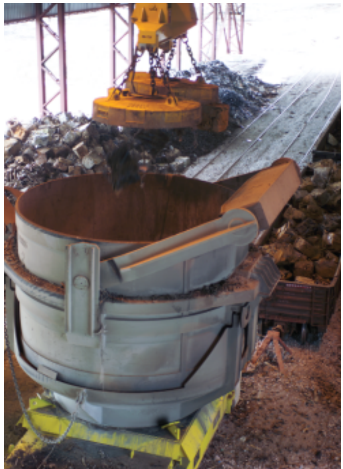
Top: The recently enclosed 100,000-square-foot storage and distribution center, where bundles of finished product will be stored and staged for shipment. Bottom right: A 30-ton electromagnetic crane moves steel scrap into a scrap bucket. Two such buckets, each containing 55 tons of recycled steel, are charged in the mill's electric-arc furnace (EAF) to produce 100 tons of molten steel. Bottom left: The bar-products mill looks out over central Indiana farmland.
