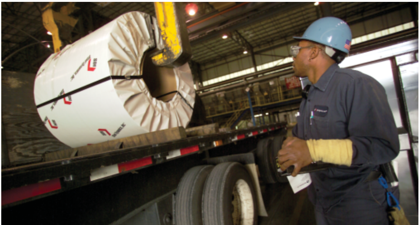
Ronnie Ellis, a shipping crane operator at SDI's Jeffersonville galvanizing plant, uses a radio-controlled crane to load a finished coil of steel onto an outbound truck. Radio operation from the floor allows the operator to better view the crane and control its load, providing a greater margin of safety.
