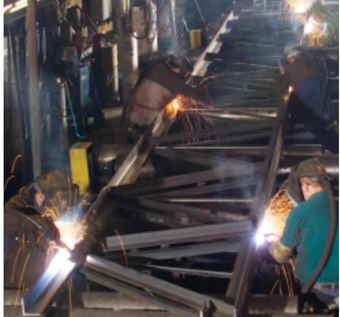
A highly efficient team of welders quickly fabricates a large joist at the New Millennium plant. Many of the welded joists' steel components are roll-formed from flat-rolled sheet steel supplied by SDI's Flat Roll Division.
