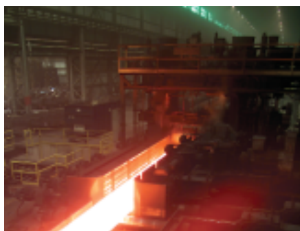
Top, left to right: The process of rolling wide-flange beams is controlled by tandem-mill operator Doug Gilliam, who sits in a “pulpit” high above the beam’s path as multiple rolling passes are made; a bundle of finished structural steel—in this case, H-piling—is retrieved by a heavy-duty lift-truck for shipment. Bottom, left to right: The first step in rail production is a sequence of 11 passes through the roughing mill to reduce a rectangular bloom to a rough-rail shape; metallurgist Ken Reid and rolling-mill supervisor Bob Johnson check rail dimensions during an October production trial; and a glowing rail section, resting on its side, speeds from the finishing mill to the hot-cut-off saw.
