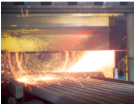
Top, left to right: Foundations are set for the new eight-stand rolling mill to be installed in the spring of 2004; unfinished bars "walk" across the large-product cooling bed before being cut to length. Bottom, left to right: A circular abrasive saw slices through a row of round bars; continuous hot-steel strands exit the caster to be cut into blooms for rolling; and Rob Kibler, a rolling-mill supervisor, "sizes" a hot bar to ensure that it meets dimensional specs.
