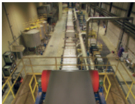
Top, left to right: Hot-rolling a steel slab to produce thin-gauge hot-rolled sheet steel in SDI's seven-stand hot mill; glowing flat-rolled steel is down-coiled onto a mandrel, from which it will be removed as a coil of steel—a hot band. Bottom, left to right: A view from the entry-end of Butler's new paint line, which is over 1,000 feet long; workers adjust the flow of paint to the rollers in the paint-application room; and various colors of painted coils, banded but not yet wrapped, await shipment.
