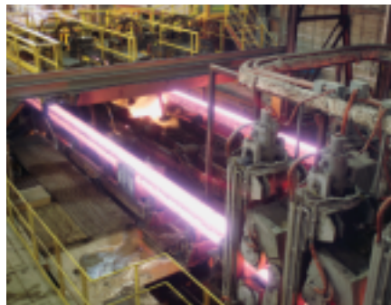
Top, left to right: Foundations are set for the new eight-stand rolling mill to be installed in the spring of 2004; unfinished bars "walk" across the large-product cooling bed before being cut to length. Bottom, left to right: A circular abrasive saw slices through a row of round bars; continuous hot-steel strands exit the caster to be cut into blooms for rolling; and Rob Kibler, a rolling-mill supervisor, "sizes" a hot bar to ensure that it meets dimensional specs.
