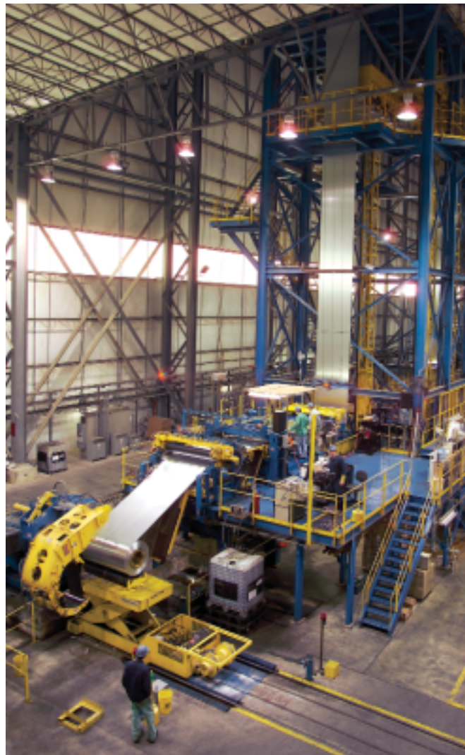
Left: A cold-rolled steel coil, banded for shipment. Such coils can be sold as is or galvanized (on Butler's Galv Line 2 or at SDI's newly acquired Jeffersonville galvanizing facility). Right: The final inspection and coiling station at the Jeffersonville galv line illustrates the new plant's highly automated equipment, similar to that used at Butler.
